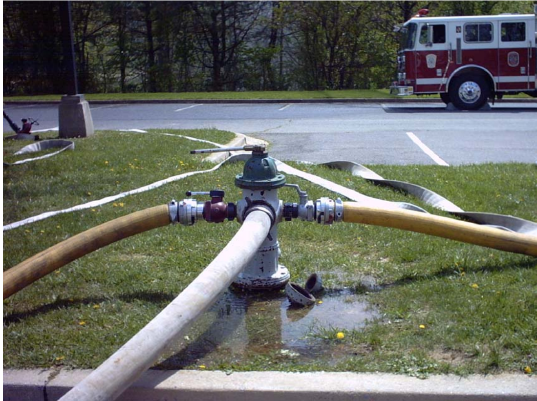
A real heavy water hookup – and the hydrant was still not maxed out!
