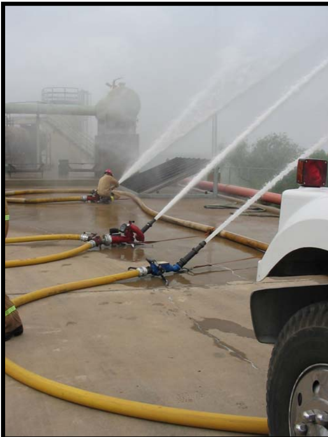
“2,064 gpm through three portable monitors. Unknown volume through the pre-piped monitor.”
