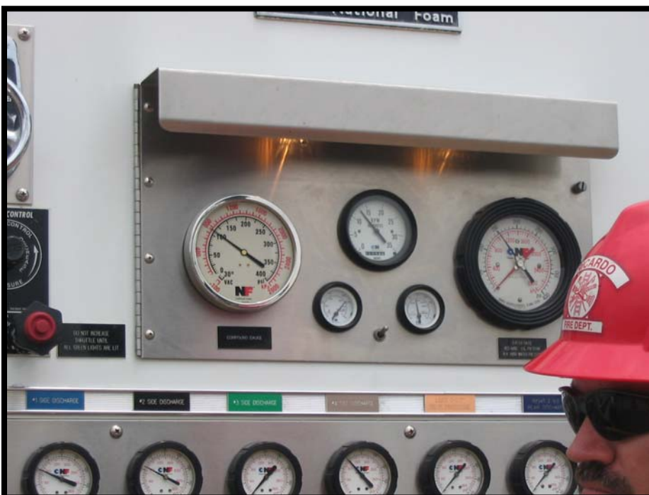
“A residual pressure of about 100 psi is recorded while flowing the 2350 gpm. Wow!!! Literally more water than what this rig could get rid of.”
