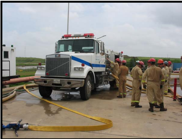
“The set-up – two, 5-inch lines feed this 1500 gpm foam pumper as the pumper supplies three, portable monitors.”
